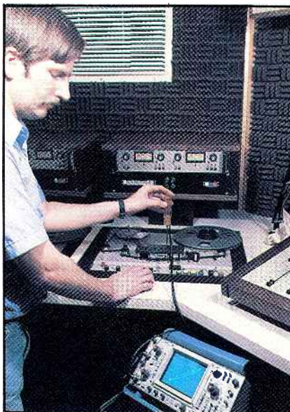
Reel-to-reel tape machines should be checked on a regular basis for top performance. The results of each set of measurements should be kept on file as a means of detecting developing problems in a particular machine. KANU engineer Jerry Hetherington checks one of the station's recorders.
